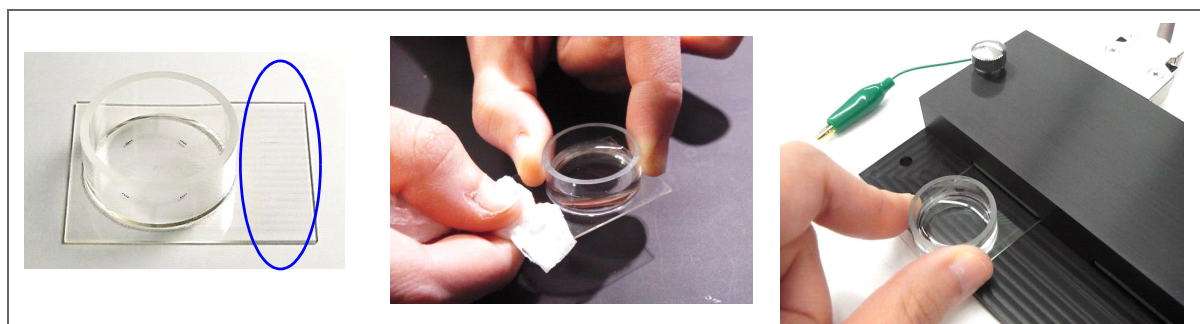
Figure 13. Terminal for the MED Probe 16 (left, marked with blue), cleaning its terminal (middle), and installing the MED Probe 16 onto the MED Duet Connector (right).
